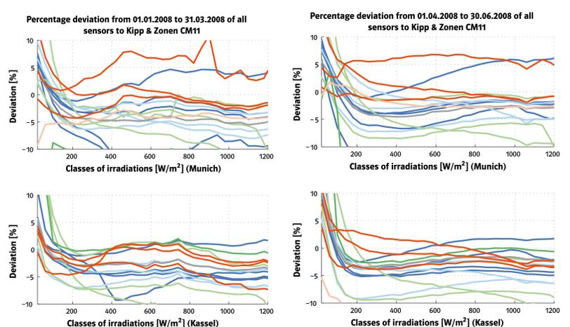
**Figure 5:** In these diagrams for the two locations and the individual quarters of the year 2008 the proportional deviations for the individual irradiation classes are represented.
