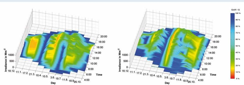
**Figure 1** illustrates the diurnal variations of the weather situation at the selected reference days at the two locations Munich (on the left-hand side) and Kassel in a four dimensional graph. As fourth dimension over the colouring a statement is integrated to the diffuse radiation fraction of the irradiation performance.
