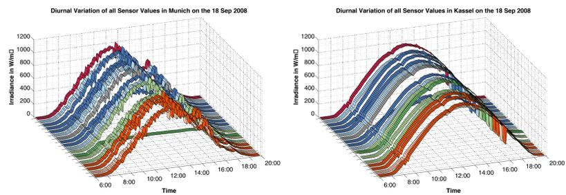
**Figure 2** shows the diurnal variations of both reference installations, the operational performance of the individual sensors on one single exemplary day (on 18. September 2008). Not absolute values are of intent but the sensor behavior relatively to each other gives an impression to the usability of individual sensor instantaneous values and the importance of knowledge about the deployed sensors.
